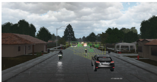
Figure 4. Simulating pedestrian crossing the road while on cell phone. Simulation done in VIRES VTD.
